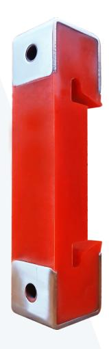
EasyGrip Sound Furring Clip resiliently secures common drywall furring channel Offering significantly higher STC values than drywall attached to resilient channel, EasyGrip ensures that installers will not inadvertently screw through the "resilient" leg of the channel into the joist or stud.
