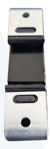
EasySound Furring Clip resiliently secures common drywall furring channel Offering significantly higher STC values than drywall attached to resilient channel, EasySound ensures that installers will not inadvertently screw through the "resilient" leg of the channel into the joist or stud.
